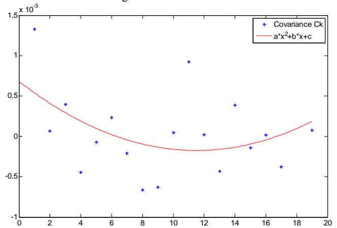
**Figure 4: Calculated covariances  $C_k$  per counter  $k$  for boresight misalignment angle  $\omega$  and the fitted curve  $C(r)$ .**
