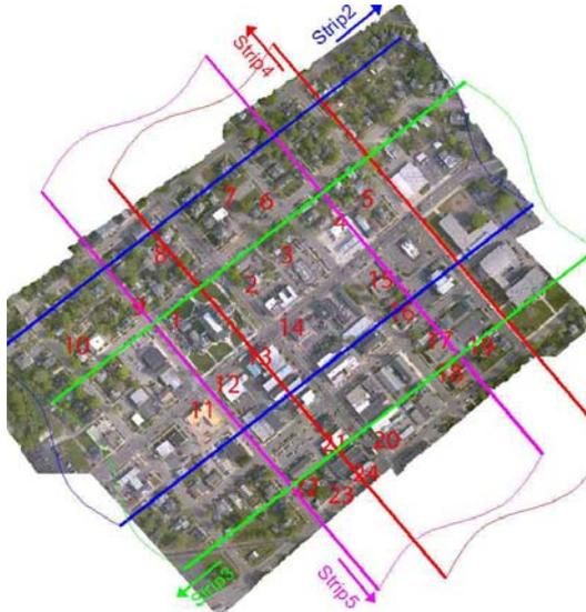
**Figure 3: Highlighted (numbered) buildings distributed in the area and LiDAR strips' orientation**
