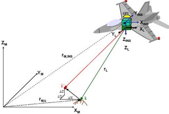
Figure 1. LiDAR system components
