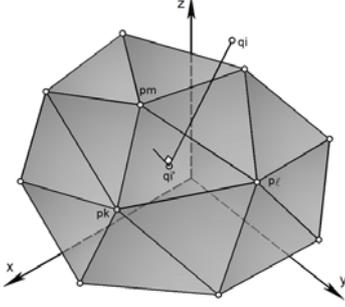
**Figure 4.** Point  $q_i$  is a point of surface Q that is transformed to surface patch of P surface as  $q_i'$ . The shortest distance from  $q_i$  to the surface is used for determining the 3D transformation
