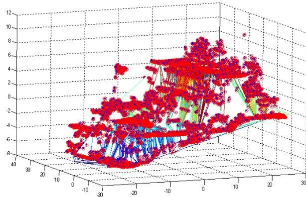
Figure 7. Photogrammetric restitution (highlighted TINs), LiDAR points are shown by blue circles (before) and by red circles (after the convergence) (e.g. Project 2)
